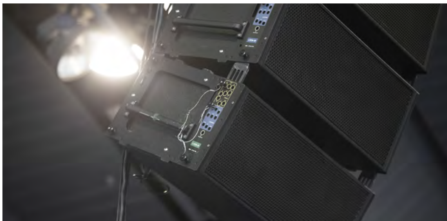
Line array loudspeaker used to distribute sound
